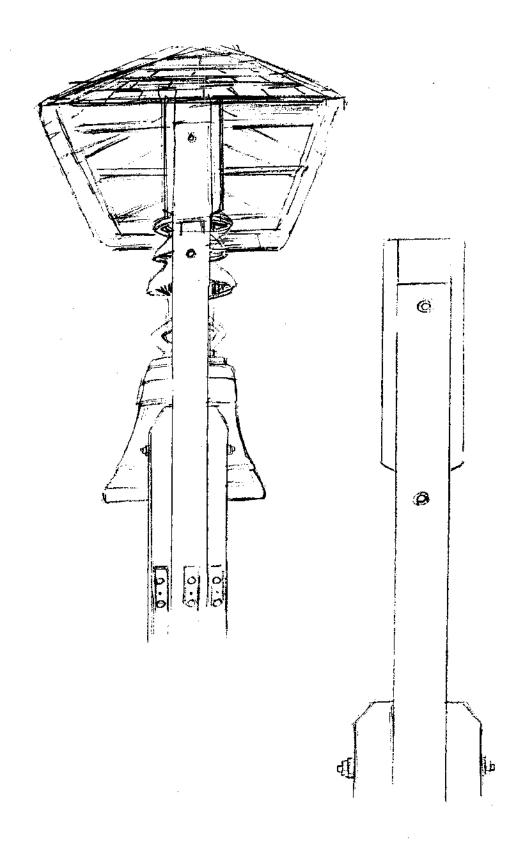
This is how the footers are made. In our climate, it is desirable not to set a wooden beam directly into the ground because the dampness of the soil will inevitably cause the beam to rot.
